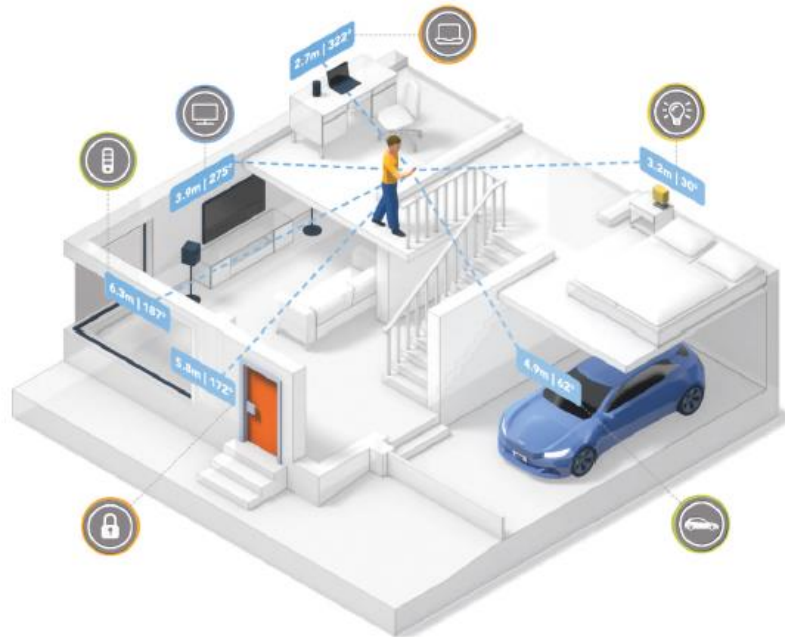
Figure 1: NXP Trimension™ - Use of UWB radio technology as a distance and direction sensor in a smartphone, a vehicle and the Internet of Things
